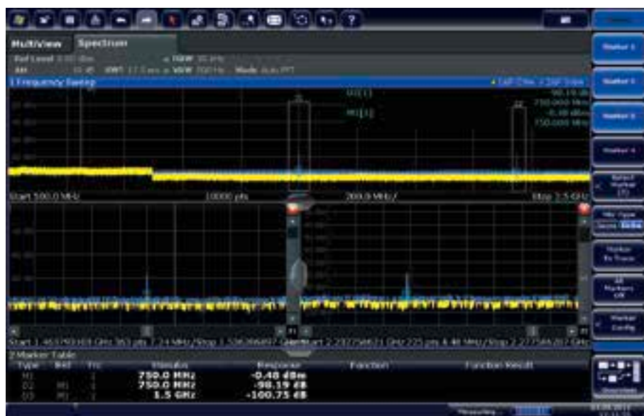
Harmonic measurement with highpass filter on (yellow trace) and off (blue trace).
