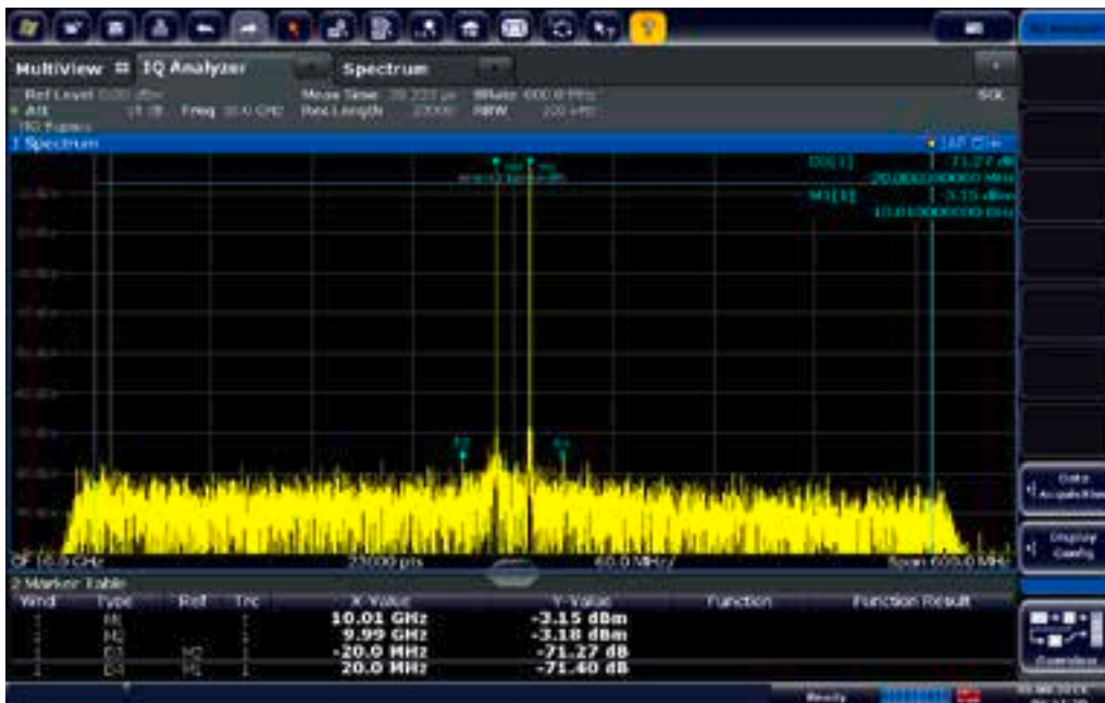
Third Order Intermodulation Distortion (IM3) of -65 dBc.
